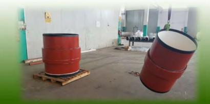
ERAM Technologies supplies pipeline Monolithic Isolation Joints for both onshore and offshore projects. Saving in the overall cost of the corrosion control system is just one of the benefits of using an Isolation Joint.
